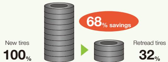
Comparison of the amount of petroleum resources needed to manufacture new truck and bus tires compared to retread tires
