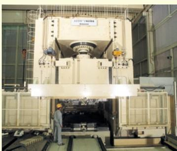
Our special Biaxial Tester, which can apply a vertical force of up to 3,200 tons, was used for the testing of large-scale seismic isolation rubber bearing used in high-rise buildings.
