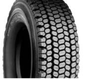
VSW is the first of its kind in snow radials, especially developed for machines used in snow removal work. This tire has excellent traction from a standing start and during acceleration as well as superior cornering and braking performance, especially on icy, packed or soft snow surfaces. VSW provides allseason service, requiring no replacement during summer and offers exceptional ability to be retreaded.
