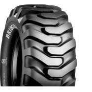
FG's separate lugs are tapered for greater traction and self-cleaning, resulting in better driving on heavy dirt and in mud.
