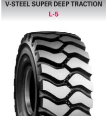
Extra-deep tread for excellent traction, comfortable ride, superior cut resistance and long tread life. The wide tread is our concept to minimize sidewall cuts. For use in underground mines, open pits and quarries.
