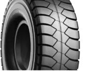
Extra-deep tread pattern with sidewall protectors. VZTP focuses especially on traction, extra-long tread life and superior cut resistance. Narrow center tread grooves, which reduce tread block movement and help with heat dissipation, along with wider side lugs, achieves the perfect balance of opposing performance targets: traction, tread life, and heat resistance. VZTP can be the best solution for large, rigid dump trucks working on muddy surfaces.
