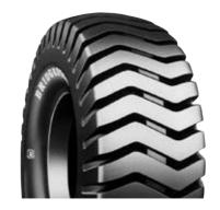
RLS's deep specially compounded rubber resists cutting and overheating. Designed for operating on rock, coal and earth surfaces where serviceability and tread cutting are problems.
