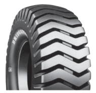
RLS's features are long tread life, thanks to extra-deep tread. Unique rubber compound resists cutting and wearing on smooth surface. Suitable for empty container handlers.
