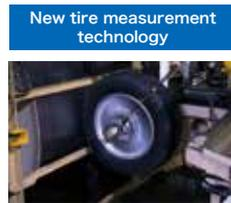
Bridgestone's proprietary technology allows the dynamic behavior of the tire in actual riding conditions to be reproduced and visualized in order to verify actual performance that cannot be understood through simulations alone.
