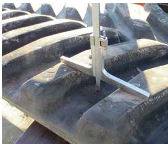
Fig. 1. How to measure the tread depth
