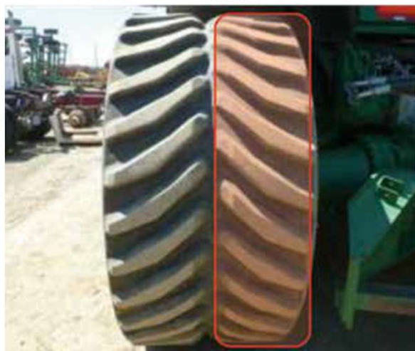
Fig. 1. Accelerated machine side tread wear
