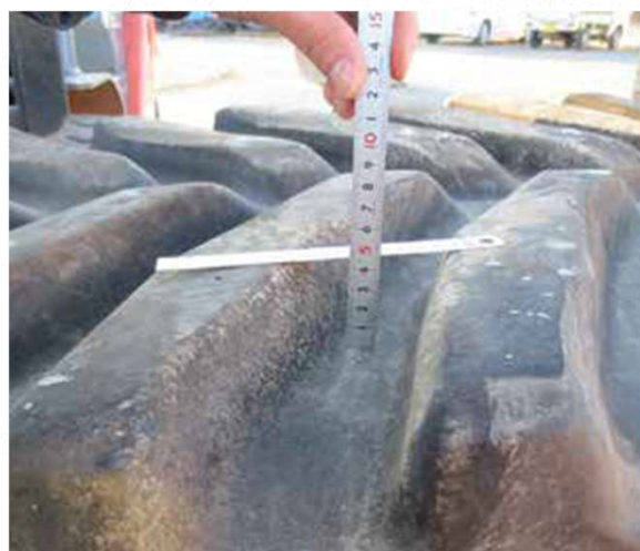
Fig. 1. How to measure the tread depth
