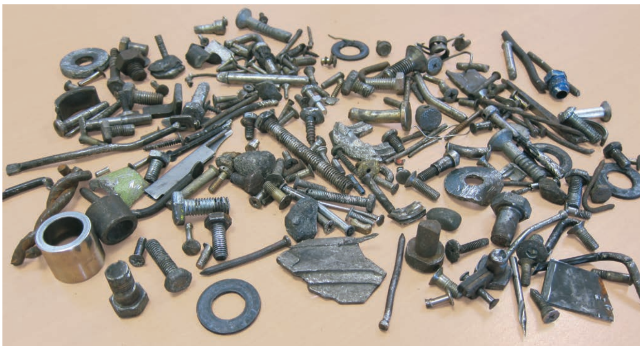
The items in the photograph were picked up from taxi ramps, service areas and runways. These objects present a potential danger to tires and to aircraft.
