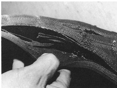
An example of Casing Break Up (CBU) in a bias tire at the lower sidewall caused by running the tire at pressures below those recommended.
