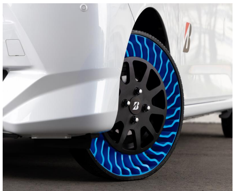
AirFree, “Next-Generation Tire” that doesn't need air-filling
