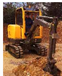
Excavator with rubber tracks
