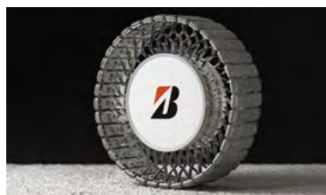
Concept model of a lunar rover tire using AirFree technology
