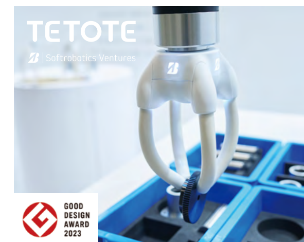
TETOTE A soft-robotic hand capable of precise piece-picking, made possible through the integration of AI software from partner Ascent Robotics.
