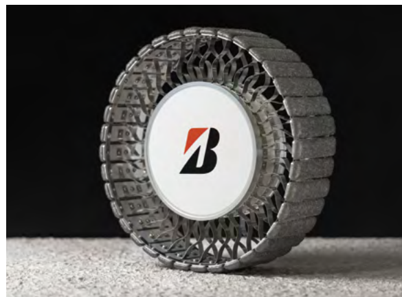
Concept model of a lunar rover tire using AirFree technology
