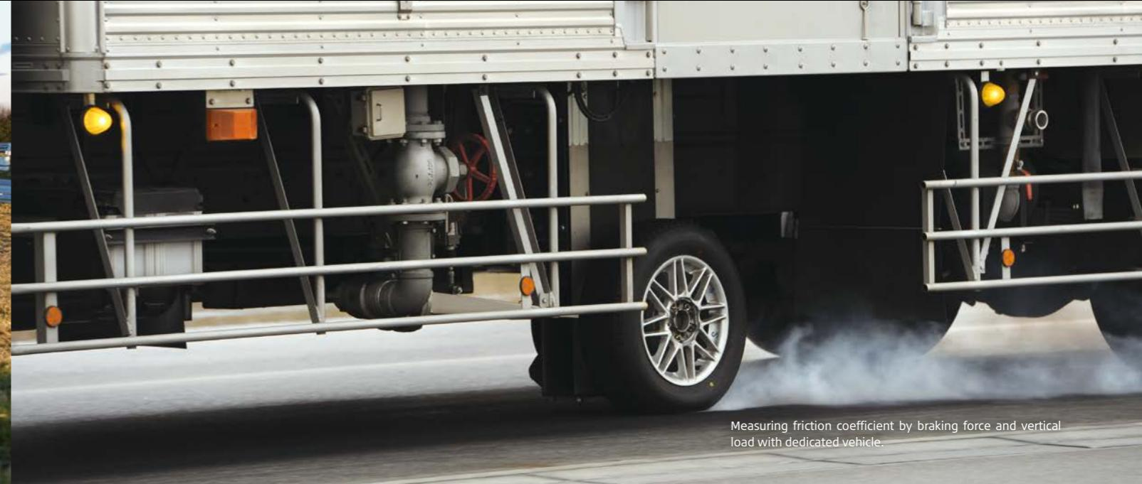
Measuring friction coefficient by braking force and vertical load with dedicated vehicle.
