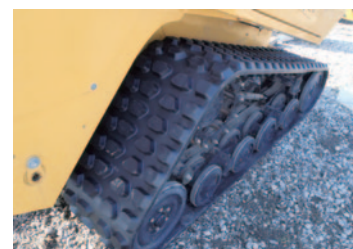
Special rubber tracks for decontamination work
