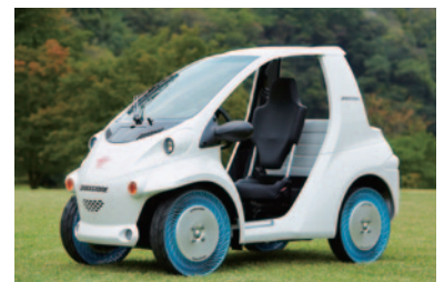
“Air Free Concept Tire” fitted to an ultralight mobility vehicle
