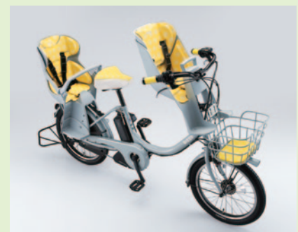
The three rider-compatible “bikke” electric-assisted bicycle
