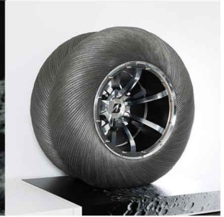
An unprecedented air-free tire with steel wool
