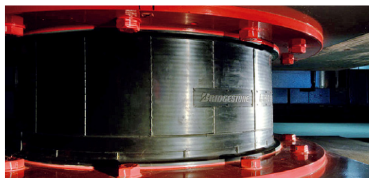
Elastomeric seismic isolation bearing
