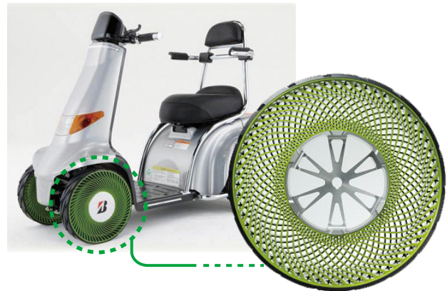
Air Free Concept Tire equipped electric carts for seniors and people with disabilities
