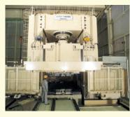
Our special Biaxial Tester, which can apply a vertical force of up to 3,200 tons, was used for the testing of large-scale seismic isolation rubber bearing used in high-rise buildings.
